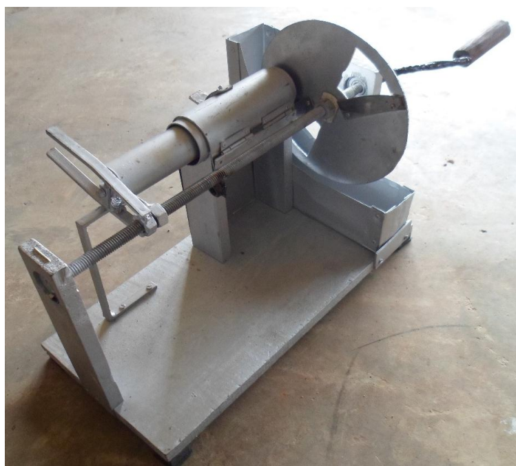
Plate 1: The fabricated hand-operated semi-automatic chopping machine
