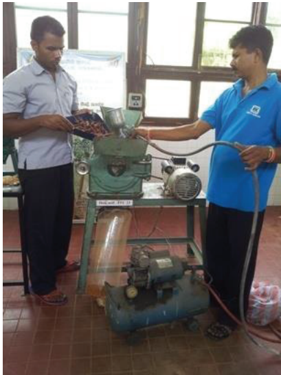
Figure 1 - Machinery set up for atomized water spraying during grinding
